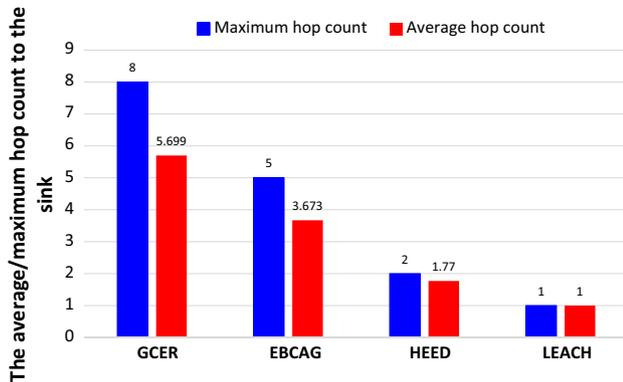
Fig. 12 The average and maximum hop count of sensor nodes to the sink
