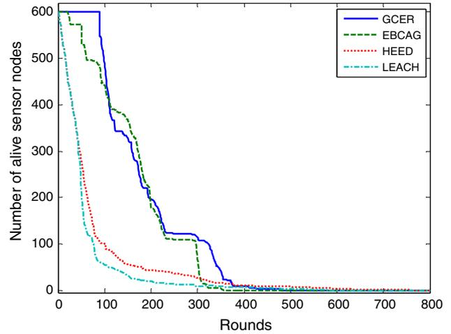
Fig. 9 Number of live sensor nodes over the time
