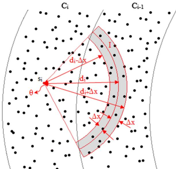
Fig. 2 The selection range of the candidate relay in the next ring by a cluster-head in the *i*th ring
